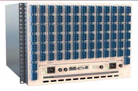
HC-S320 optical switch supports matrix all-optical switching ports, adopts MEMS (micro-electromechanical system) technology to intelligently manage single-mode optical fiber signals. This includes establishing connections, monitoring optical signals, and changing connections independent of data transfer rates and protocols. Any input fiber can be connected to any output fiber without any restrictions and obstacles.
