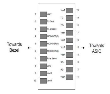
Figure 2. Pin out of Connector Block on Host Board
