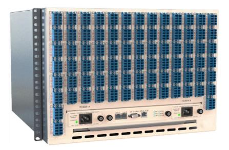
HC-S320 optical switch supports matrix all-optical switching ports, adopts MEMS (micro-electromechanical system) technology to intelligently manage single-mode optical fiber optical signals, and changing connections independent of data transfer rates and protocols. Any input fiber can be connected to any output fiber without any restrictions and obstacles.
