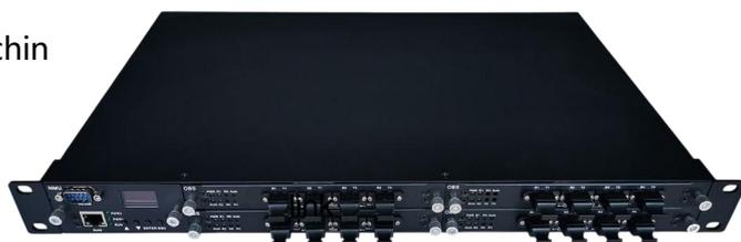
OBP - Bypass protection system is a kind of light is applied to optical fiber communication field and can automatic bypass fault intelligent network node system, through the automatic identification of the network node power supply system and optical signal output state, when the node fault system, automatically instantaneous switch, light path around the fault of network nodes, so as to avoid network node all resistance barriers, maintain system connected to normal.
